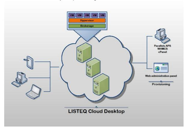
LISTEQ Cloud Desktop's architecture comprises of server(s) running a hypervisor and the Virtual Machines (native hypervisor is Oracle VirtualBox). It runs on top of the native I/O layer of the hypervisor (not using any client agents or VM RDP stack), therefore LISTEQ Cloud Desktop can support any OS running within the hypervisor. Running VMs based on Windows, Linux, ChromeOS, DOS, Mac OS X and even Android x86 are possible.
