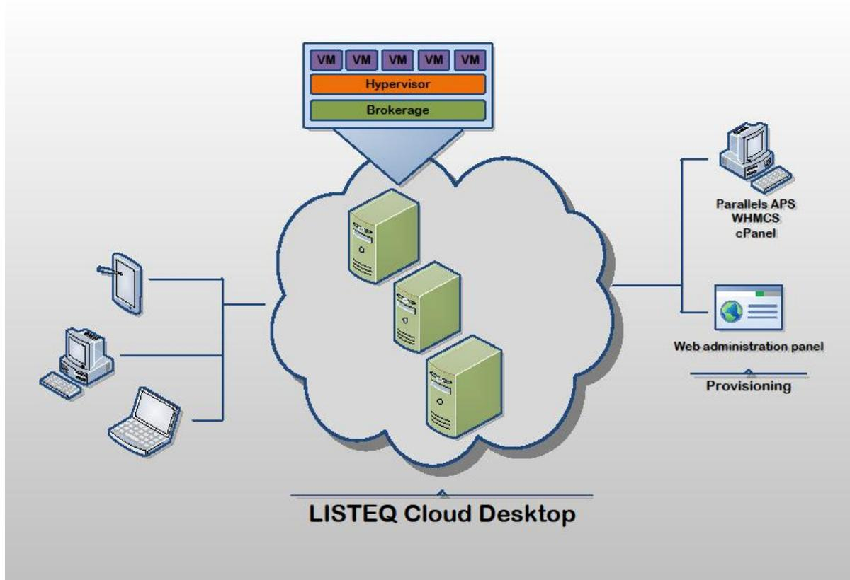
LISTEQ Cloud Desktop's architecture comprises of server(s) running a hypervisor and the Virtual Machines (native hypervisor is Oracle VirtualBox). It runs on top of the native I/O layer of the hypervisor (not using any client agents or VM RDP stack), therefore LISTEQ Cloud Desktop can support any OS running within the hypervisor. Running VMs based on Windows, Linux, ChromeOS, DOS, Mac OS X and even Android x86 are possible.
